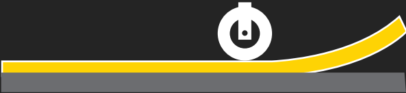
Roller tightly compresses the sound absorber
